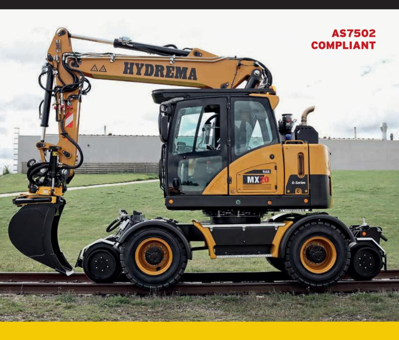
Specially designed compact excavator in the 20t class for railway work with focus on great stability, high performance and flexibility.
