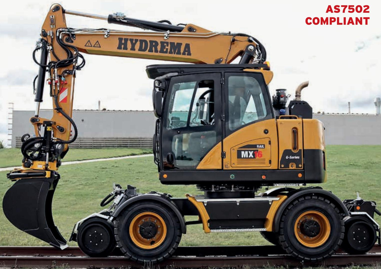
Specially designed compact excavator in the 19t class for railway work with focus on great stability, high performance and flexibility.
